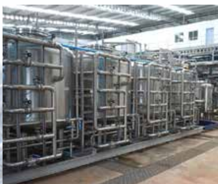
Heat sanitizable carbon filter for taste/odour removal in brewery WTP
